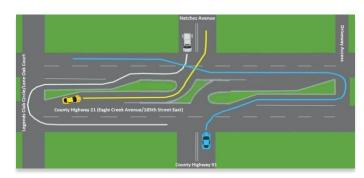
The J-turn concept is a reconfiguration of the traditional intersection that is used to improve traffic flow. It is being used in many locations across Louisiana. It is a method that safely and efficiently manages high traffic volumes at intersections with multiple approaches along a divided highway. The J-turn functions by redirecting through- and left-turning traffic on the side street approach to turn right proceed to the nearby U-turn and then return to its original
