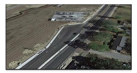
A *loon* is an expanded paved apron opposite a median crossover. The purpose is to provide additional space to facilitate the larger turning path of a commercial vehicle along narrow medians.
