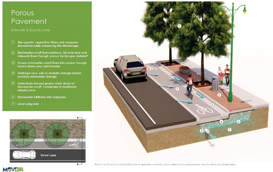
Figure 11-2: Porous Pavement Typology
