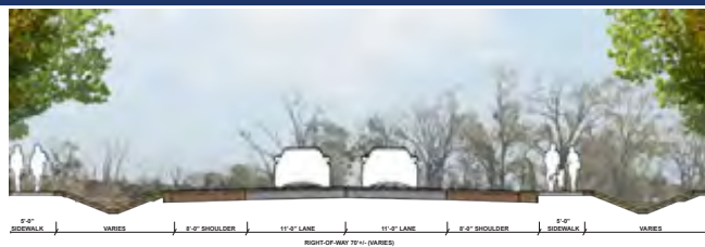
Typical Section AA - Proposed Improvements (LA 964 TO PIN OAK SUBDIVISION) Not To Scale
