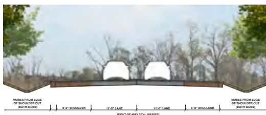
Typical Section BB - Proposed Improvements (PIN OAK SUBDIVISION TO LA 19) Not To Scale
