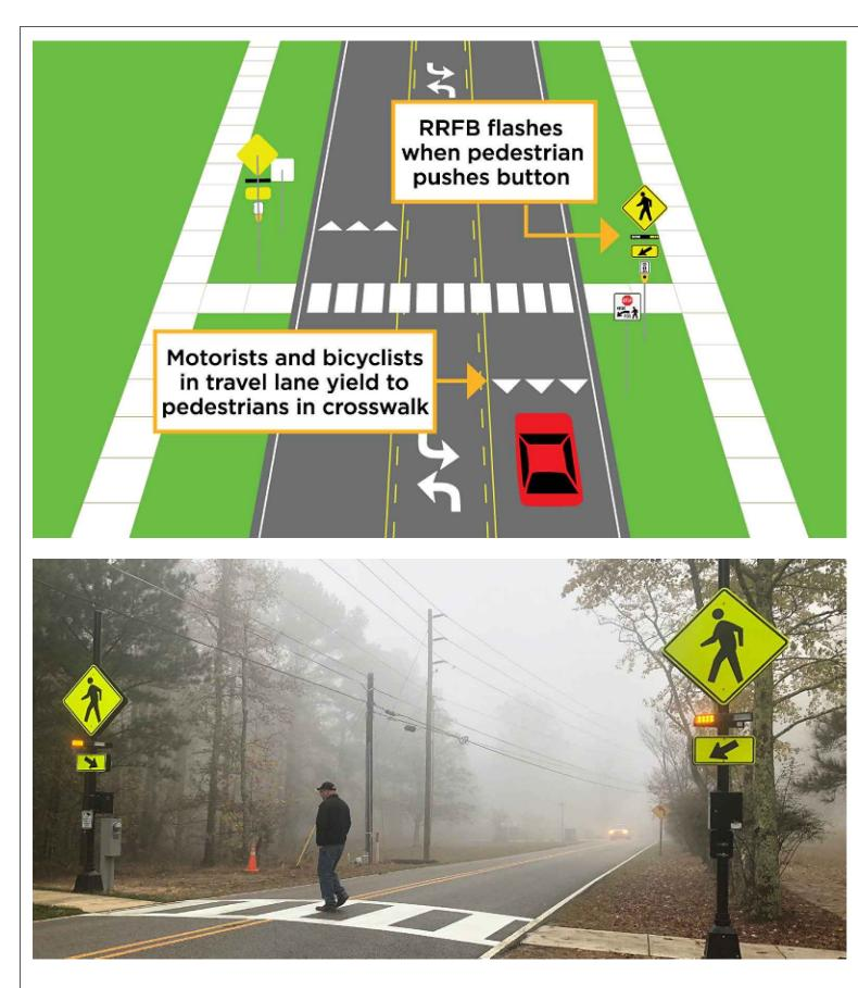
Rectangular Rapid-Flashing Beacons (RRFBs) are pedestrian-activated traffic control devices used in combination with a pedestrian, school, or trail crossing warning sign to improve safety at uncontrolled, marked crosswalks.
