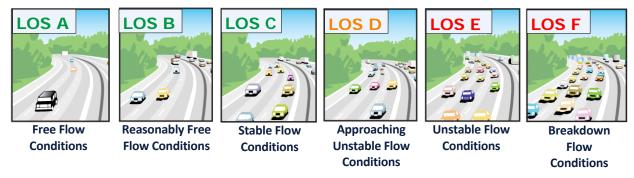
Figure 4. Traffic Level of Service Conditions
