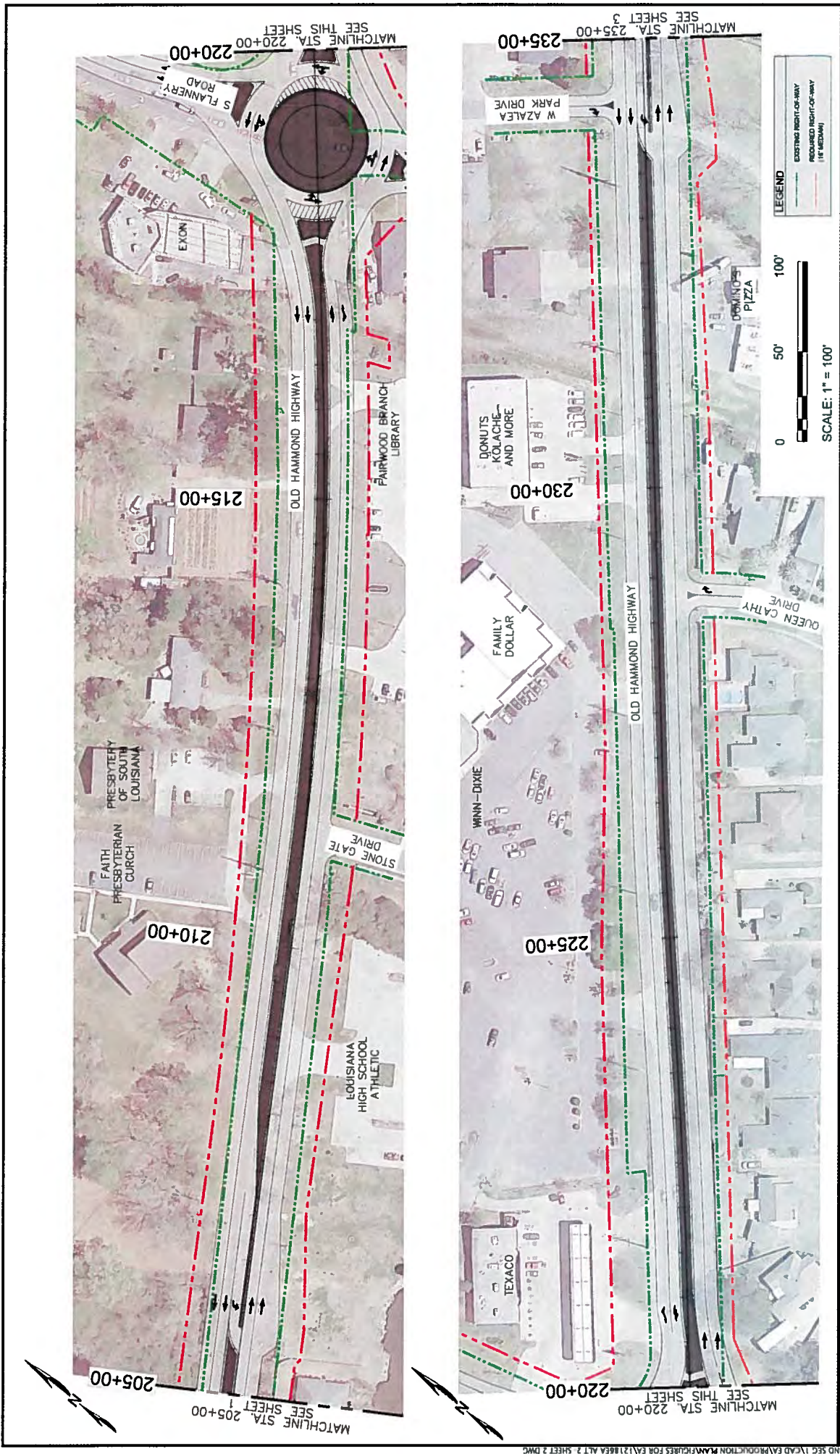
FIGURE 8 SHEET 2 OF 3 BUILD ALTERNATE 2 (16' MEDIAN WITH 2 ROUNDABOUTS)
