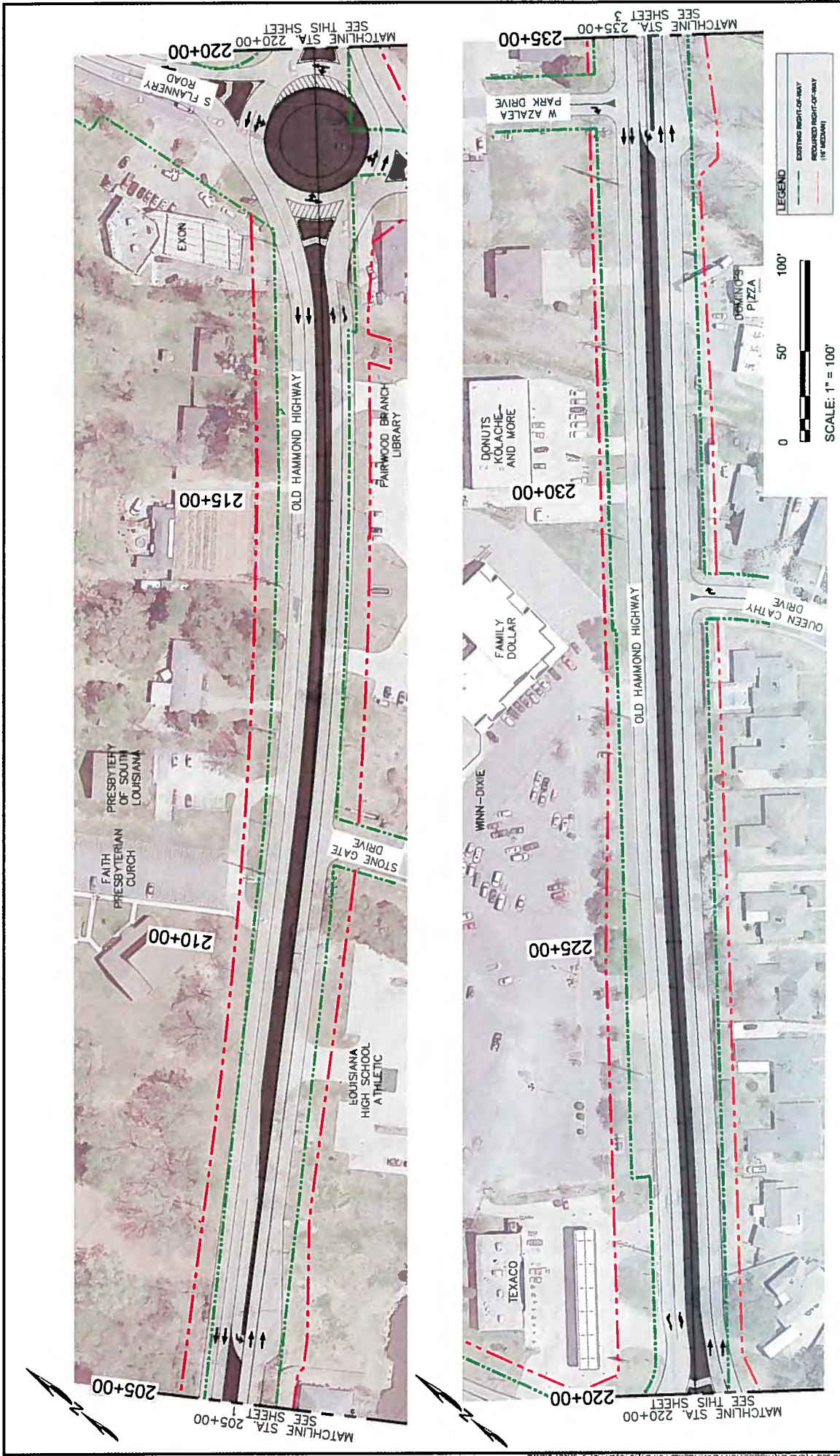
FIGURE 9 SHEET 2 OF 3 BUILD ALTERNATE 3 (16' MEDIAN WITH 1 ROUNDABOUT)
