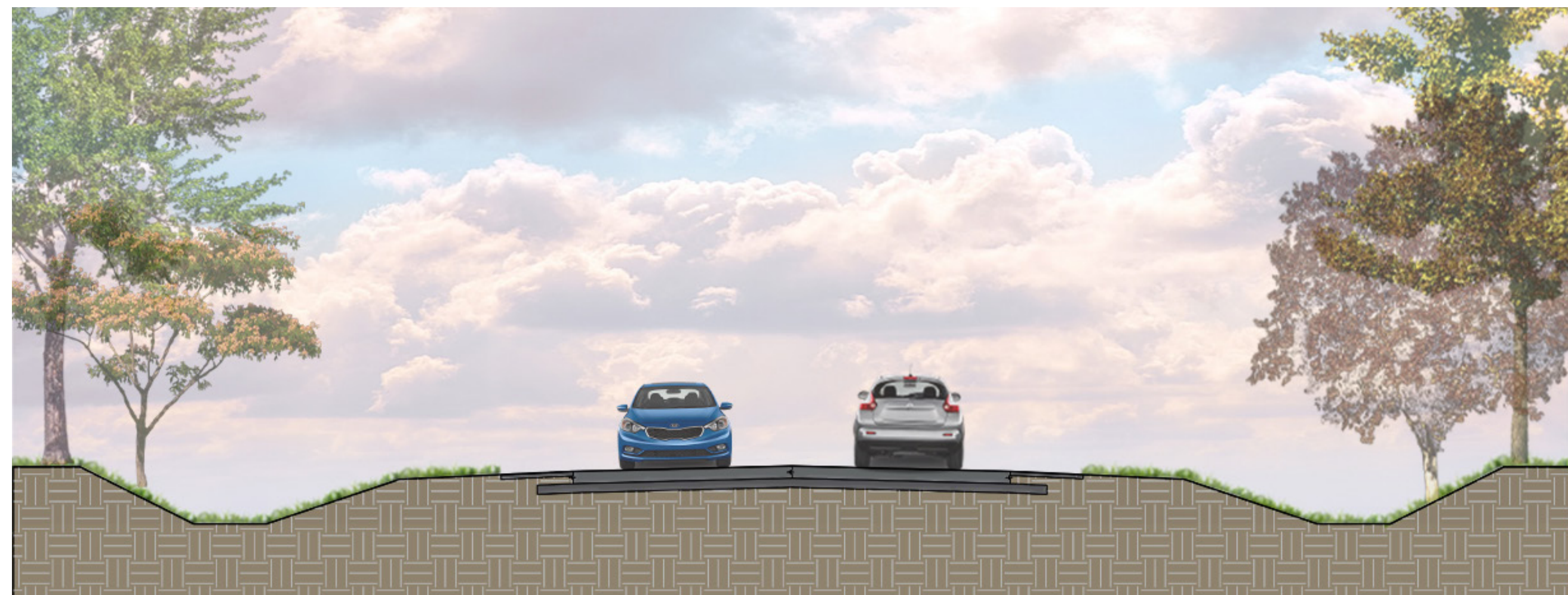
Open Ditch for Stormwater Management Shoulder 12'+/- Travel Lane 12'+/- Travel Lane Shoulder Open Ditch for Stormwater Management
