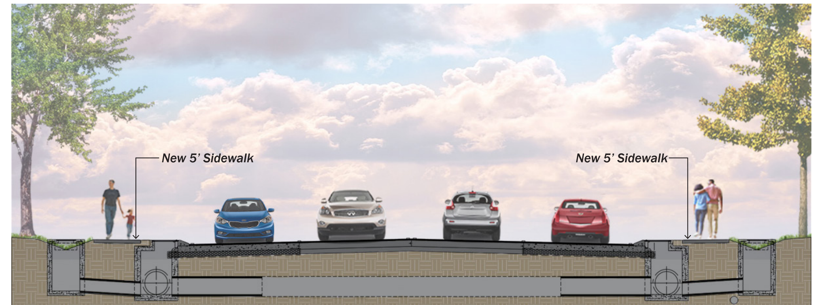
Subsurface Stormwater Management New 5' Sidewalk New 12' Travel Lane Existing 12'+/- Travel Lane Existing 12'+/- Travel Lane New 12' Travel Lane New 5' Sidewalk Subsurface Stormwater Management
